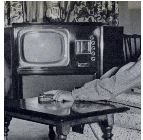
This 1954 HOWTO from Mechanix Illustrated invites the reader to take apart the family TV set to make a remote-controlled mute button (called a "SHADDAP")
